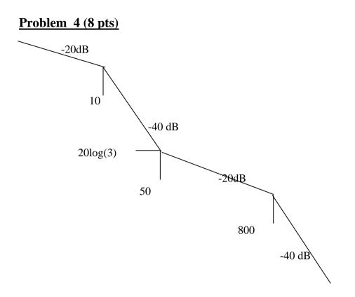
The asymptotic gain versus frequency of the open minimum-phase transfer function is shown for a unity feedback control system. a. Obtain the open-loop transfer function, (2 pts)
